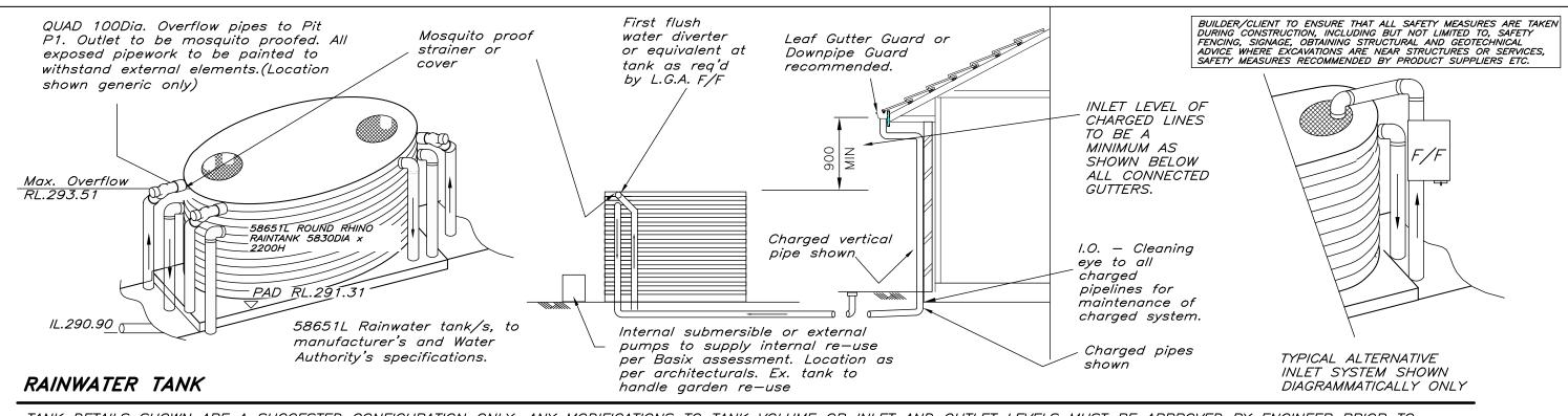
TANK DETAILS SHOWN ARE A SUGGESTED CONFIGURATION ONLY. ANY MODIFICATIONS TO TANK VOLUME OR INLET AND OUTLET LEVELS MUST BE APPROVED BY ENGINEER PRIOR TO COMMENCEMENT OF CONSTRUCTION. TANK SHAPE, & DEVICES SHOWN ARE DIAGRAMMATIC ONLY. MINIMUM OF 450 CLEARANCE (UNLESS L.G.A. REQUIRES LARGER SETBACK) TO SIDE BOUNDARIES MUST BE MAINTAINED. CLIENT IS RESPONSIBLE TO ENSURE COMPLIANCE WITH THIS IN THE INSTALLED STATE. Charged stormwater lines from Roof Areas ONLY to rainwater tank.
